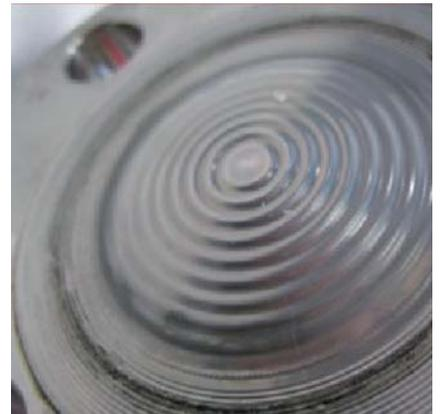
A pressure instrument with Diaphragm Seals is filled under high vacuum at a temperature of +/- 20 °C. When the instrument with Diaphragm Seals is being used at an operating temperature different to this, a measurement error will occur.
